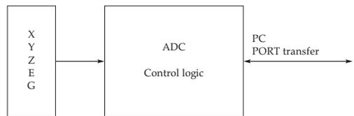
**Figure 3.** Principle of the Slovenian acquisition system. Positional, strobe, energy and gate signals are converted into digital form in the acquisition card, which sends them to the computer through PORTs without interrupt service.
